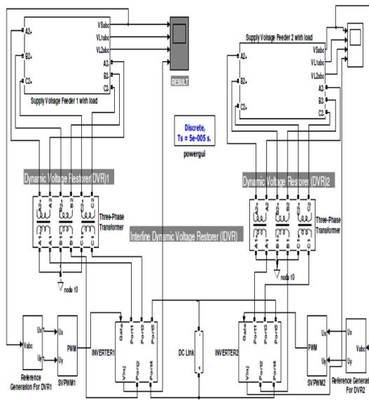
Fig.6. Simulation of IDVR system based on SVPWM technique
