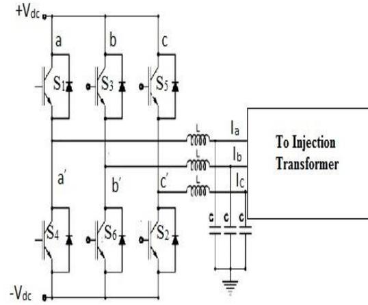
Fig.2. Three-leg voltage source inverter
