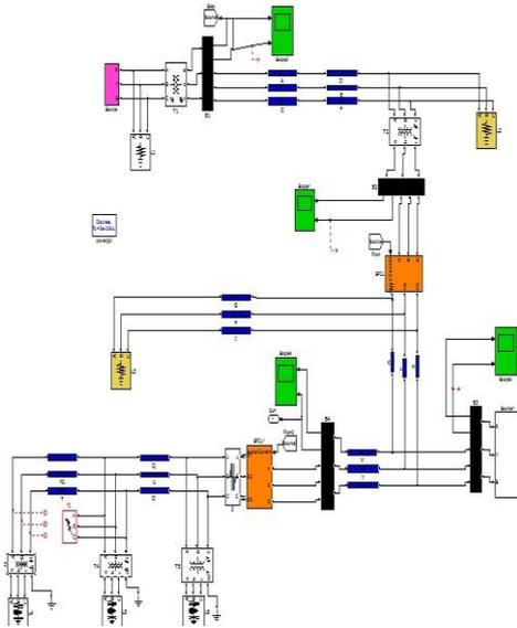
Fig. 7 proposed SFCL system with SFCL
