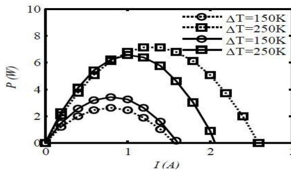
Figure No.1: Effects of temperature dependence on power versus electrical current [1]
