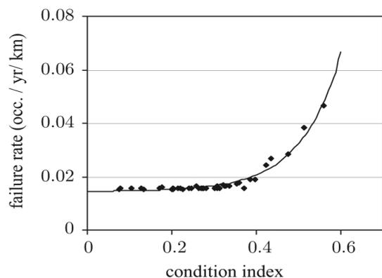
Fig.16: Relation of condition index and failure rate of overhead lines [1].
