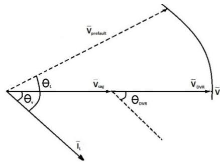
Fig.5 In Phase Compensation Method
