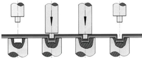
Fig.4: Principle of mechanical clinching
