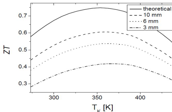
Figure no. 8:- The modules  $ZT$ -values versus the cold-side temperatures  $T_k$  for different leg sizes. The simulations predict, that modules with longer legs show a better performance [3].
