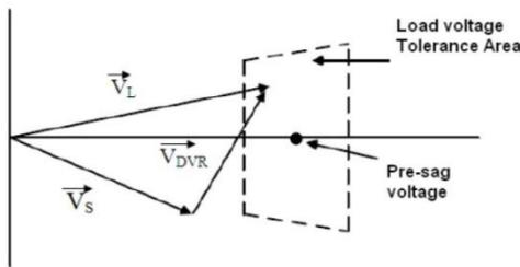
Fig.6 Voltage Tolerance Method
