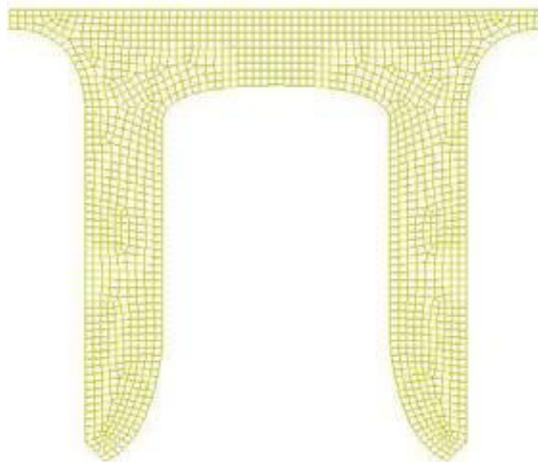
Fig.13 – Simulation geometry of Rivet
