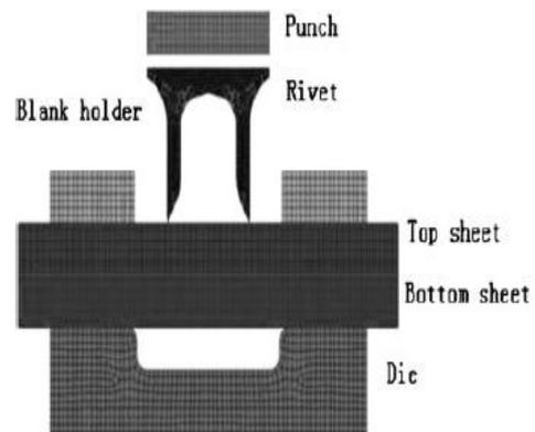
Fig.7.- FE model of SPR process
