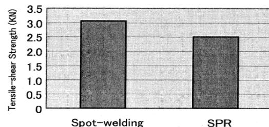
Fig.5- Tensile-Shear strength comparison of Spotwelding and SPR
