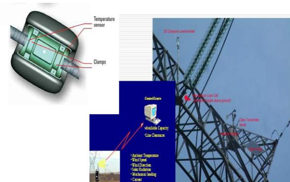
Fig:8 Monitoring System version 2 ( OTLM) Monitoring system provides real-time monitoring of temperature and current on OHL [10].
