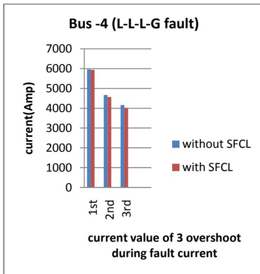
Graph.4: Fault current at bus 4 with SFCL and without SFCL
