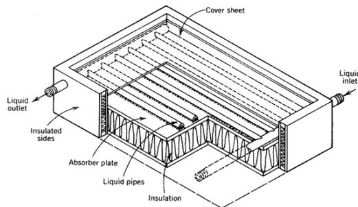
Flat-plate collectors are used for residential water heating and hydronic space-heating installations.
