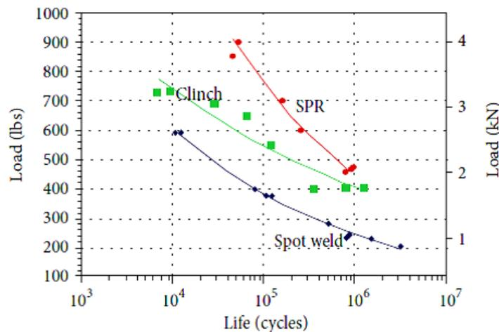
Fig.2 Fatigue behavior comparison of SPR, clinch, and spot-weld joints
