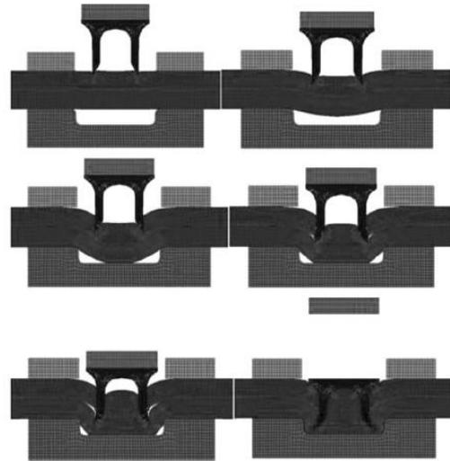
Fig.8 Simulation of SPR process
