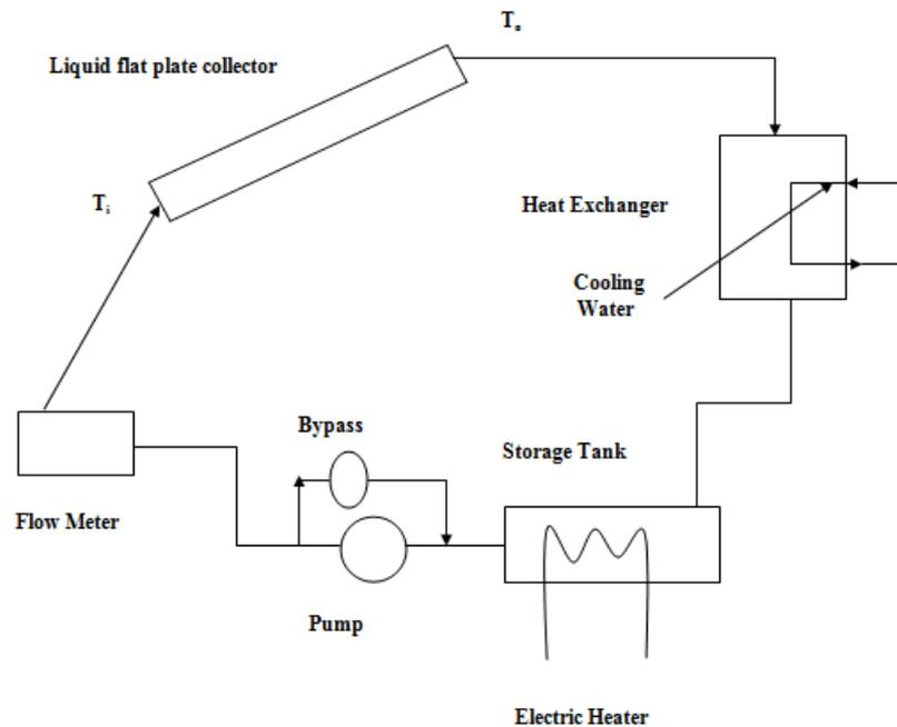
Figure 2 Closed loops set up for testing flat collector
