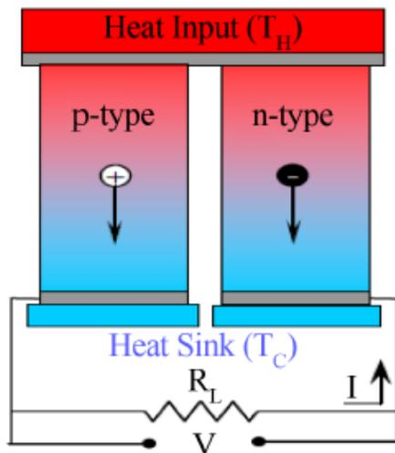
Fig. Arrangement of thermoelectric module for power generation by seeback effect
