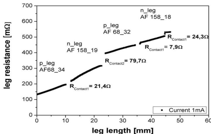
Figure no. 9:- The discontinuities represent the contact resistances, the linear slopes the resistance of the thermoelectric legs [3].
