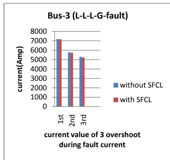
Graph.3: Fault current at bus 3 with SFCL and without SFCL
