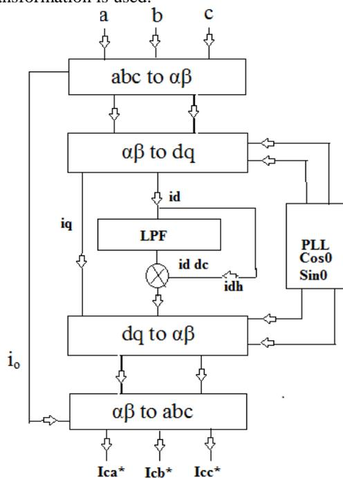
Fig No.2 Block diagram of SRF based algorithm
