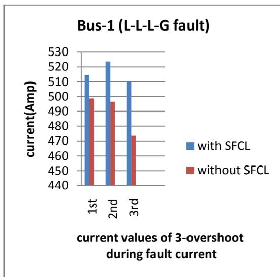
Graph.1: Fault current at bus 1 with SFCL and without SFCL
