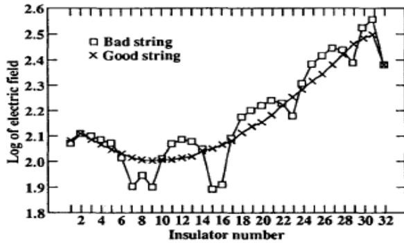
Fig: 6 Log of electric field Vs Insulator no. [10]
