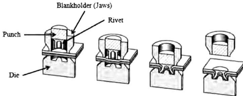
Fig.1.SPR Operation with semi tubular Rivet
