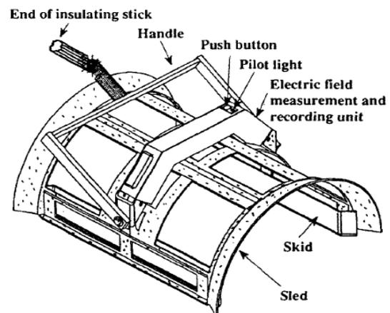
Fig: 5 Insulator tester [10].
