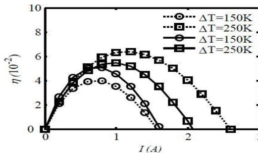
Figure No.2: Effects of temperature dependence on efficiency versus electrical current [1]
