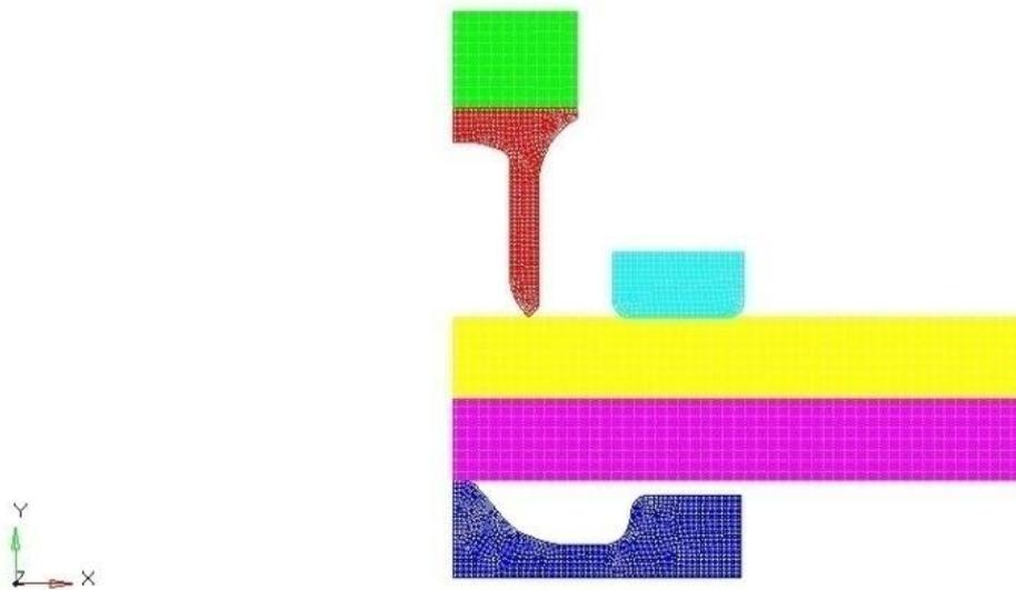
Fig. 9– FE Model for SPR Process
