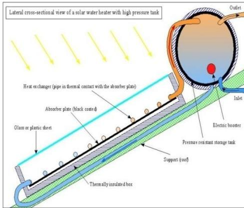
Fig-Basic Structure of SWH
