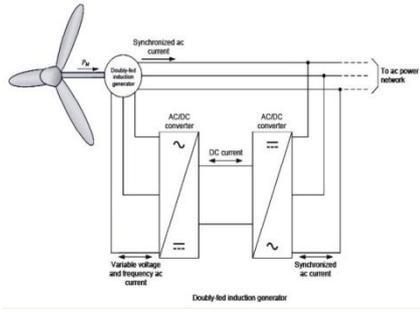
Fig.1 DFIG wind turbine block representation
