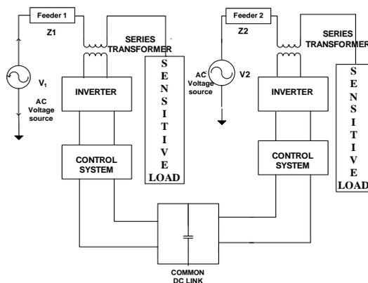
Fig.1. Interline dynamic voltage restorer
