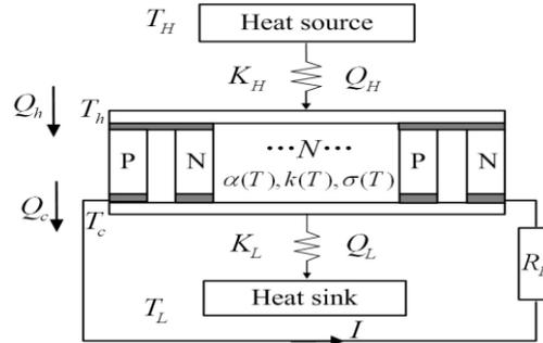
Figure 1:- The finite time thermodynamic model of an irreversible multi-element thermoelectric generator with external heat transfer. [2]
