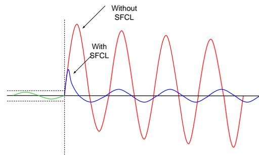
Fig.1: Fault current waveform with SFCL and without SFCL
