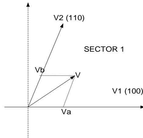
Fig.5. Reference voltage generation in sector one space vector
