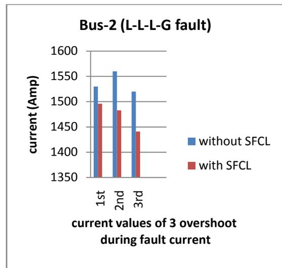
Graph2: Fault current at bus 2 with SFCL and without SFCL
