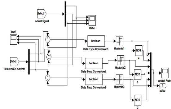
Fig No. 4 Simulation diagram of hysteresis current control
