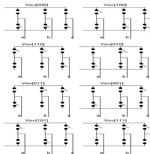
Fig.3. eight switching states of inverter
