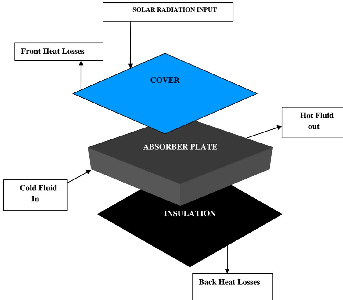
Figure 1: The Flat Plate Solar Collector
