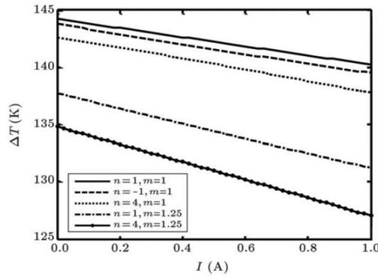
Figure No.6: Effect of heat transfer law on temperature difference versus working electrical current. [2]
